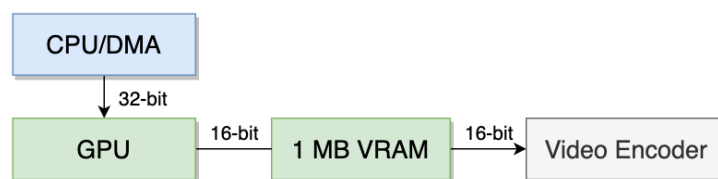
Figure 3.24: Graphic layout of the VRAM
