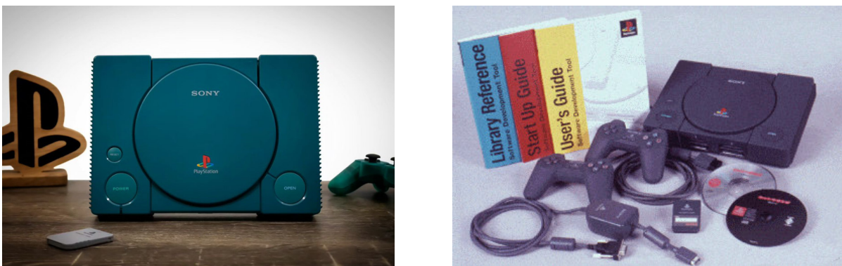
Figure 3.13: On the left, the DTL-H1202 Debugging Station model. On the right, the Net Yaroze DTL-H300x kit
