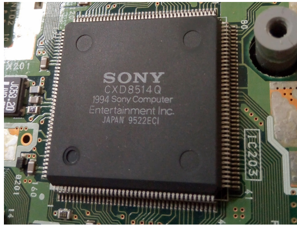
Figure 3.23: Graphics processor (GPU) used in the SCPH-100X series of the Sony PlayStation [35]
