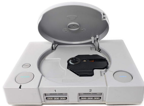
Figure 3.7: The position of the optical reader has been changed compared to previous models [22]
